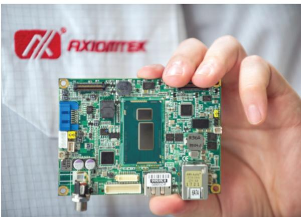
Axiomtek mitigates the difficulties encountered with hardware design and allows the SkySpecs technology team to focus on software development required to make the inspection service possible. Axiomtek's smallest form factor, Pico-ITX, has been one of the leading industrial motherboards in the market.
